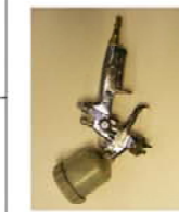
for smaller spray jobs small gravity feed gun
